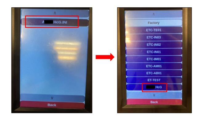
Step5. Press the profile you would like to put into the reader. \*Can only do one profile at a time\*
